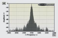
ABOVE: Wow and flutter re. 3150Hz tone at 5cm/sec (plotted ±150Hz, 5Hz per minor division). Absolute speed is very accurate indeed
